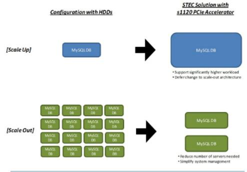
Figure 3: MySQL Server Consolidation with STEC Solution
